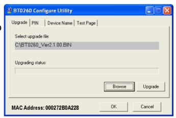
In the process of upgrading, other buttons are disabled and you are not able to close this application until it finishes.
