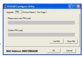
The maximum length of PIN code is 16 bytes containing any printable characters.
