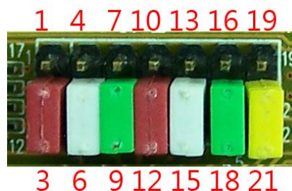
7 x 3 header block to enable Termination and BIAS resistors
