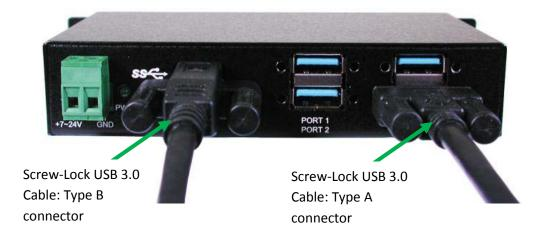
Self Power Input Connector: This 2-pin (one pin for positive voltage and the other pin is GND) terminal block connector is used to connect strong power to self-power the hub, the voltage can be in the range from +7V to 24VDC.
