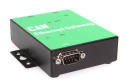
The NCAN-1 is designed to make a fast, simple way to communicate with CAN bus devices. The NCAN-1 adds one industrial CAN bus channel to your host system with a transparent virtual serial port without limitations on operating systems and distances.
