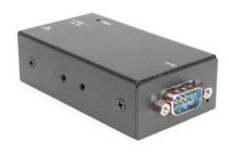
The MSD-SRP1XM-PRO is a multi-protocol RS-232 / 422 / 485 3-in-1 serial device server that is designed to connect RS-232, RS-422 and RS-485 serial devices including POS, barcode readers, sensors, meters, weighing systems, CNC controllers and PLC to an IP-based Ethernet Network.
