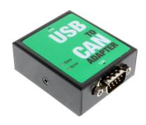
This USB to Controller Area Network device (CAN) adapter installs and is automatically recognized by your operating system. It has +/-16kV ESD protection for all signals and supports CAN 2.0A and CAN 2.0B. No external power is needed to run your CAN applications as the device runs from USB bus power
