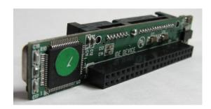
The 44P-SATA is a 2.5? 44Pin IDE Hard Drive to SATA adapter for Laptop hard drives. The 44Pin IDE (PATA) to SATA converter can be used in applications such as small form factor computers, point of sale equipment and industrial computers.
