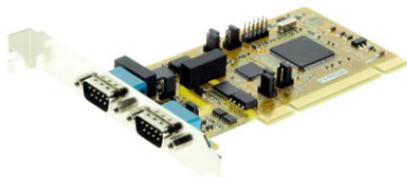
The SG-PCI2S422485IS 2 port PCI RS422 /485 Card with isolation and surge suppression maintains backward compatibility with your PCI applications and drivers to provide a scalable, high-speed serial I/O bus. Protects serial devices from ESD (Electrostatic Discharge) occurrences during operation.
