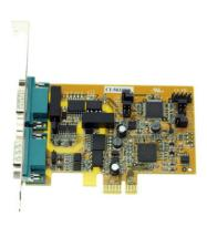
The SG-PCIE2S422485IS 2 Port RS422 RS485 PCI Express card is designed for easy installation for PC, Work Stations, Thin Client or Server serial applications. Instantly provides 2 DB9 ports for additional serial communication and adds Optical Isolation and Surge Protection to your devices.
