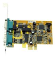
The SG-PCIE2S422485IS 2 Port RS422 RS485 PCI Express card is designed for easy installation for PC, Work Stations, Thin Client or Server serial applications. Instantly provides 2 DB9 ports for additional serial communication and adds Optical Isolation and Surge Protection to your devices.
