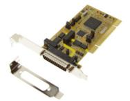
The SG-PCI2S422485OCTIS 2 Port PCI RS422 RS485 card with Breakout Cable supports low profile form factor and is designed to work with your PC, workstation, thin client, or server and provides instant 2 Port PCI RS422 / 485 Serial communication via the PCI bus already in your computer.
