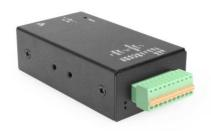
The MSD-SRP2XM-TBPRO is a multi-protocol RS-232 and RS-422 / 485 serial device server that is designed to connect RS-232, RS-422 and RS-485 serial devices including POS, barcode readers, sensors, meters, weighing systems, CNC controllers and PLC to an IP-based Ethernet Network. The MSD-SRP2XM-TBPRO provides 2 ports, port 1 supports RS-232 mode only and port 2 supports RS-422 / 485 modes.
