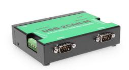
The USB-2CAN-M provides a cost-effective solution for customers to enable communication with CAN bus devices. The solution designed using an ARM Cortex-M0 32-bit micro controller and the USB to serial chip makes it very flexible in handling small burst of CAN frames at a high speed.
