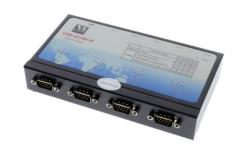
A 4-Port RS-422, RS-485 adapter for serial communication that utilizes four external DIP switches for easy access to the signal used. Automatic transmit and receive control for 2-wire RS-485 half-duplex mode.
