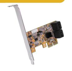
The 4 Port SATA3 RAID PCIe Cards High transfer rate is supported up to 1,000MB/S (2 lanes) for large imaging data file applications with the CG-PCIeS3-i4p. Breaking the bottleneck and extending the bandwidth while supporting HyperDuo modes is a great feature in this PCIe Card.
