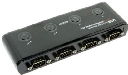
The USBG-4FTDI-B 4-Port USB to Serial RS-232 Adapter for newer computers and laptops that no longer include host serial port connection. Supports 4 new serial DB-9 connected devices through a host USB port to act as a portable Serial Bus.
