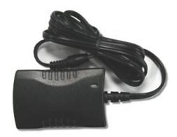
5 Volt 2 Amp output, 110v-240v auto switching external power adapter used with Coolgear hubs and Active USB cables.
