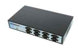
Industrial Grade Rack Mount 8 Port USB RS-232, RS-422, RS485 Octal Serial Adapter with Metal Case and Built-In 100-240Volt Power Supply utilizing a FTDI chipset.
