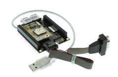
BeagleBone I/O Module with automatic recognition of USB ports and SD card when installed. Utilizes GL852G USB 2.0 MTT Hub controller to expand the single USB port connections.
