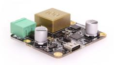
This High Power Single Port USB Type-C Industrial PCBA that complies with the latest USB-C and PD standards. Intended for use in PC power adapters, mobile chargers, car chargers and power bank applications. This charging board provides one 100W USB Type-C PD port.
