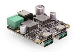
The ChargeIT! Dual Port Charger provides an effective amount of Charging power ideal for Tablets, Cell phones, and laptops. The USB PD charger board incorporates both Standard Type-A and USB PD Type-C charging ports. The wide DC input voltage range is ideal for 12V DC and 24V DC Vehicle applications.
