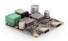
The ChargeIT! Dual Port Charger provides an effective amount of Charging power ideal for Tablets, Cell phones, and laptops. The USB PD charger board incorporates two USB PD Type-C charging ports. The wide DC input voltage range is ideal for 12V DC and 24V DC Vehicle applications.
