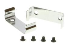
Gives DIN Rail Mounting capabilities to USB hubs, serial adapters, IP Adapters, or Ethernet servers that are designed for mounting applications. For Mounting on to a standard 35mm DIN RAIL (7.5mm and 15mm depth.)
