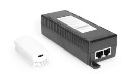
Coolgear's newest USB Type-C PoE adapter works with a Cat5/6 cable from a PoE injector connected to its RJ45 port. This extends the length of power to the Nest Cam Indoor or Nest Cam Outdoor by up to 100 meters from a power source. Use the Type-C USB port to connect the Nest Cam.
