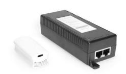
Coolgear's newest USB Type-C PoE adapter works with a Cat5/6 cable from a PoE injector connected to its RJ45 port. This extends the length of power to the Nest Cam IQ Indoor Gen 1 or Nest Cam IQ Outdoor Gen 1 by up to 100 meters from a power source. Use the Type-C USB port to connect the Nest Cam.
