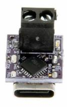
Negotiate the voltage into the USB C PD port connection with this nano sized USB PD to DC module. The module is meant for hobbyist who enjoy building their own circuits. If you've designed a board to work at a certain voltage level through a Type-C connection, this module can make sure you get the required voltage to your project
