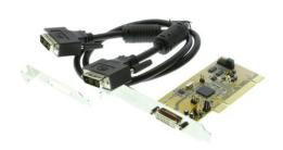
This PCI to PCIe host adapter connects from your computer system to an external expansion box source for PCI/PCIe system growth and functionality.
