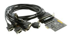
The PCI Express Add on Card supports RS232 serial connections through an octopus cable enabling 8 additional COM ports to your system through the PCI Bus. The PCI card itself uses a 62-pin cable connector to enable the 8 serial ports.
