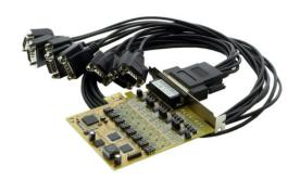
This PCIe Add on Card extends your systems RS422 or RS485 serial device connections by 8! Using this PCI Express Card interface and a DB44 to DB-9(8x) octopus cable connection enables both ESD and Surge protections to you serial devices. All cable connections are screw lock mechanisms for secure point to point contact.
