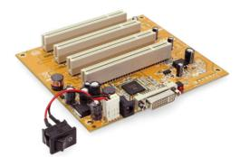
The PCI expansion board component kit gives you the option of expanding your I/O bus to an additional 4 PCI slots via the host PCIe card. All PCI slots are fully compliant with PCI Bus Rev. 2.3.
