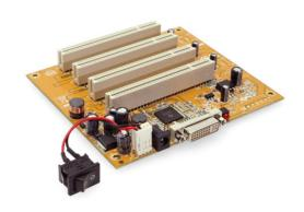
The PCI expansion board component kit gives you the option of expanding your I/O bus to an additional 4 PCI slots via the host PCIe card. All PCI slots are fully compliant with PCI Bus Rev. 2.3.
