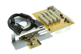
The PCI expansion kit gives you the option of expanding your I/O bus to an additional 4 PCI slots via the host PCIe card to a chassis enclosure with the included expansion board and DVI like cable and components.
