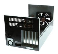
**PCI Expansion Box with Internal Power Supply**
