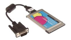
Serial Port Adapter - Host Controller Card
