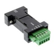
Make short work out of converting your serial port signals from RS-232 to RS-485 by using a 5-Pin terminal block converter connection. Easy to use with no drivers required, works on all operating systems.
