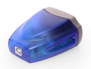
RS-422 | RS-485 | 128 Bytes Receive | 256 Bytes Transmit | FTDI
