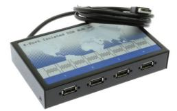
Each USB device connected to the isolated hub can operate independently. This isolated 4-port hub is designed with individual port power management. When any downstream port is overloaded or over-current, the port will shut down itself alone without affecting or terminating the normal operation.
