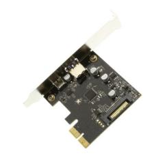
Processing 10Gbps SuperSpeed + data transmissions has become easier for Desktop, Workstation, and Servers with USB 3.1 PCIe Host Controller Cards.
