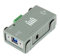
This power delivery injector USB Type-C adapter connects new USB-C technology devices to be added to legacy USB Type-B hosts.
