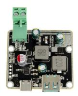
High Power Industrial PCBA using Cypress CCG2 chipset providing 60W USB Power Delivery with Type-C port, and 18W QC 3.0 with USB Type-A charging port for legacy devices.
