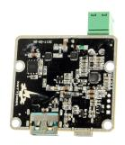
USB 60W PCBA - Type-C Power Delivery and Type-A Legacy Charging
