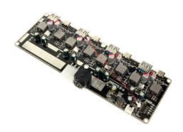
Coolgear Labs multi port USB Type-C / USB Type-A High powered charging circuit board is designed for integration into your own shell designs. Charge your laptops, add it to a charging cart or system and experience the benefits of high power charging.
