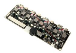
Coolgear Labs multi port USB Type-C / USB Type-A High powered charging circuit board is designed for integration into your own shell designs. Charge your laptops, add it to a charging cart or system and experience the benefits of high power charging.
