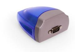
Isolated industrial USB to Serial port on USB connect RS-422 and RS485 devices, used in industrial environment. With RS-485 the data direction is controlled by the port, without further action from the software.
