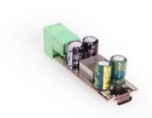
Coolgear's 24V DC with phoenix connector to USB-C PD board lets you integrate with Legacy input power to support New USB-PD devices.
