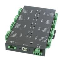
The USB2-8COMi-SI-TB is a USB 2 to 8-port industrial serial adapter that protects you device(s) with optical Isolation, 15KV ESD protection and 600W surge protection over each port. It is designed to make RS-422 and RS-485 serial port expansion quick and simple through its terminal block connection. Our series of Industrial USB 2.0 to terminal block serial adapters supports RS-232, RS-422, and RS485 electrical protection per port and are designed with the user in mind.
