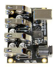
Individual hub circuit board with ESD and Surge protection over each USB port. USB 3.1 Mini 4 Port component board can be installed by itself in equipment or in different configurations for use. Compliant with USB 3.1 Gen1 with up to 5Gbps of data transfer speed.
