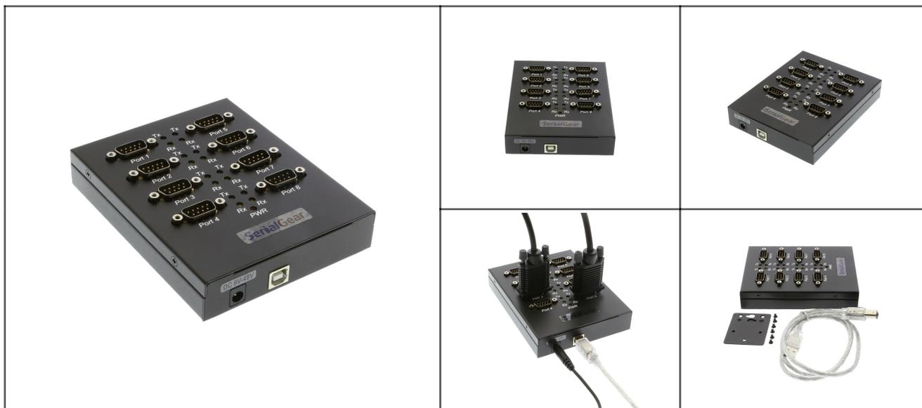
Professional Grade Solution for Legacy or Industrial serial RS-232 device connectivity to a Laptop or Desktop Computer. This Adapter Retains all COM port setting assigned by the operating system and or modified by user. This is very convenient if the adapter is disconnected and reconnected at a later time to another USB port on the same computer.
