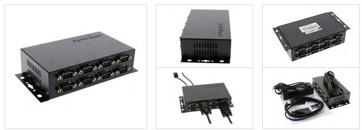
The CM-41082 is an Isolation and surge protection 8S RS232 to USB serial adapter that is designed for PC, thin client, or server to provide instant COM port expansion via the Universal Serial Bus (USB). The CM-41082 provides the scalability to quickly adapt to new USB technologies. Multiple modules can be added to a single USB interface allowing you to add RS232 connectivity as needed.
