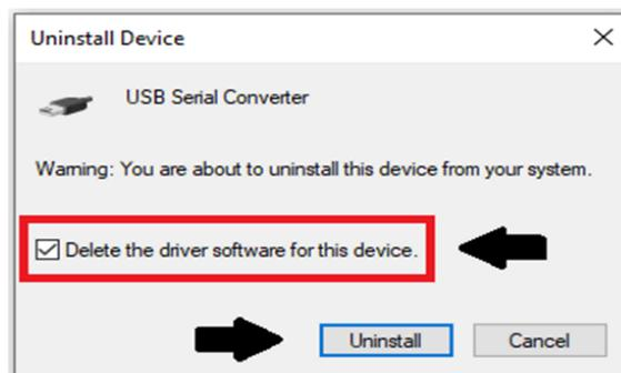
Note : If you have more than one USB Serial Converter installed in your PC, you need to repeat steps 8 - 10 to delete the driver software for each converter.
